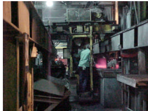
Figure 5: Tipover Operator Discharging Kiln
