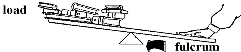
You can lift heavy objects easier by moving the fulcrum closer to the load. The load is the object or objects you want to lift. If you want to use the least amount of energy, move the fulcrum closer to the load. The longer the lever the easier it is to lift a heavier load.
