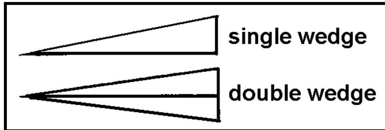
Wedges can be used to split things apart. They can cut things. The point of a nail is a wedge. A nail has a wedge point so it can go into wood more easily. The point of a screw is also a wedge. An ax blade is a wedge that splits wood apart. Other examples of wedges are: the end of a push pin, the point of a needle, the edge of a shovel and the sharp edge of a knife.
