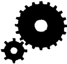
Some wheels have jagged edges. These wheels are called **gears**. Gears are special wheels with pointed edges like teeth. These pointed edges help the wheels turn each other. There are two gears on a bicycle. The large pedal gear is connected with the smaller back gear by a chain. You can find gears in watches, ice cream makers, egg beaters, and cars.
