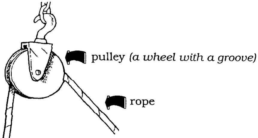
Pulleys are used in many ways. There is a pulley at the top of flag poles. Can you find the pulley at the top of the flagpole? There is a pulley at the top of a sailboat mast to raise and lower the sails. Construction workers use pulleys to lift steel beams. Pulleys are used to lift a load up, down, or sideways. Where have you seen a pulley lift something off the ground?
